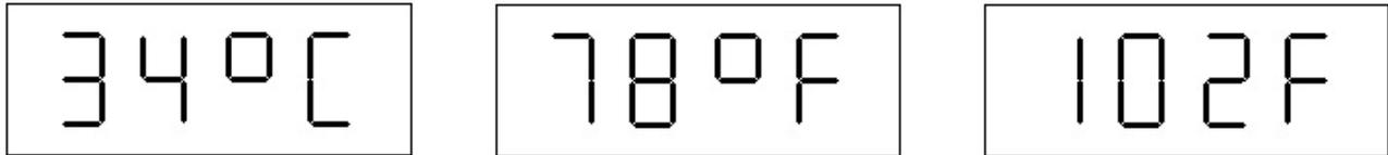
Figure 4.1 Display formats for Celsius, two digit, and three digit Fahrenheit.
