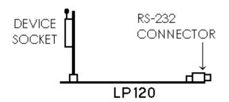
Programming-modules should be inserted or removed only when the power to the LP120 is off! As depicted in the diagram below, the programming-module should be inserted so that the programming socket faces away from the LP120 circuit board.
