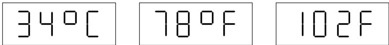
Figure 4.1 Display formats for Celsius, two digit, and three digit Fahrenheit.
